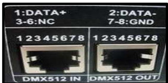
Uses RJ45 as interface signal
