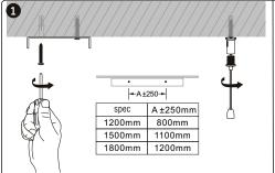
Install the ceiling bracket to the ceiling. And according to the size of the lamp, keep the distance of 2 fixed points.
