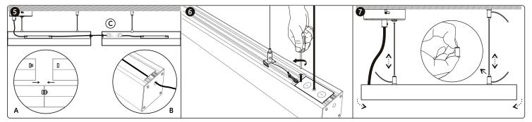
Splicing diagram, A. Connect 2 lamps with nuts. B. Cross the wire. C. Insert the terminal.
