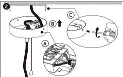
A. Connect the cable to the terminal.
