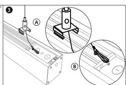
A. Fasten the stainless steel shrapnel to the lamp. B. Fasten the safety hook into the safety hole, as shown in the figure above.
