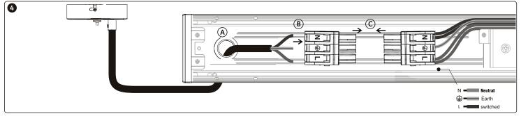
A. Insert the cable into the power hole. B. Insert the terminal into the cable. C. Insert terminals.
