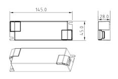
DALI dimmable DT8 CCT driver 220-240V - Output 6-54V DC - 500-1400mA - 45 W
