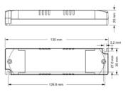
DALI dimmable DT8 CCT driver 220-240V - Output 6-42V DC - 100-700mA - 12 W
