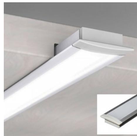
Recessed aluminum profile for LED strip with diffuser - 2 covers - 23x8mm - 2 meters
